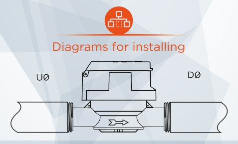
Straight sections are not necessary at the Atlantis input or output UO-DO.
